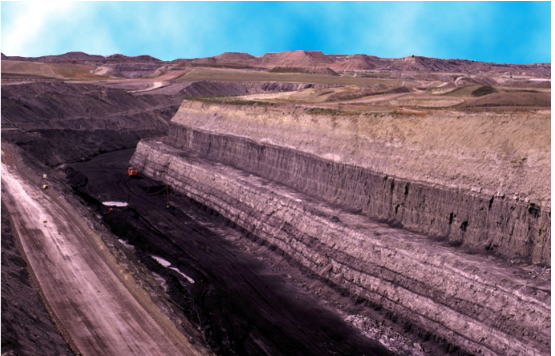
Figure PS-15. The split Wyodak–Anderson coal zone (upper bed is Anderson or Dietz 1 coal and the lower bed is Dietz 2 coal) in the Decker coal mine in Montana. The coal beds are split by tabular crevasse splay sandstone interbedded with mudstone and siltstone. Photograph by R.M. Flores.
