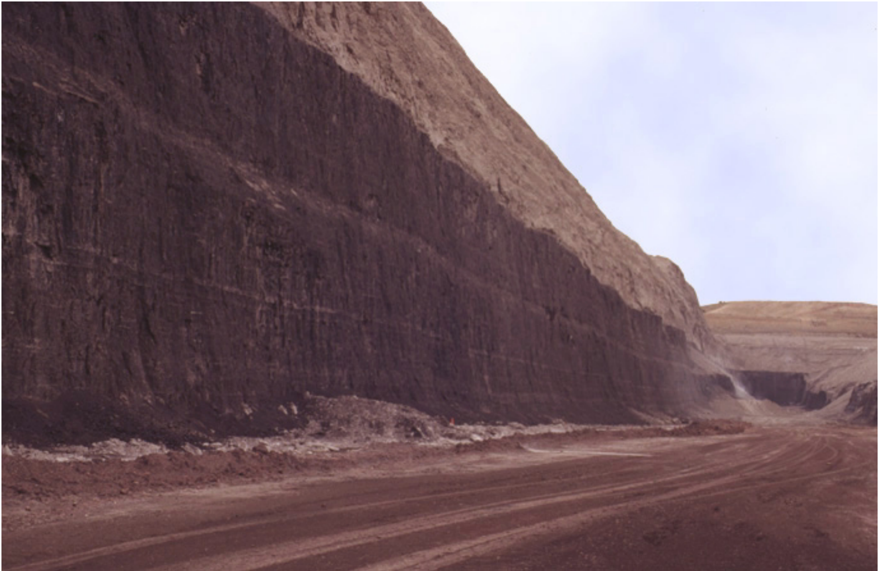
Figure PS-16. The merged Wyodak–Anderson coal, which is more than 80 ft thick, in the Spring Creek coal mine in Montana. Photograph by R.M. Flores.
